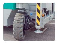
Automatic levelling outriggers for uneven or inclined terrains.
