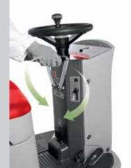
The brush head and the squeegee are lowered/raised by simply using two levers
