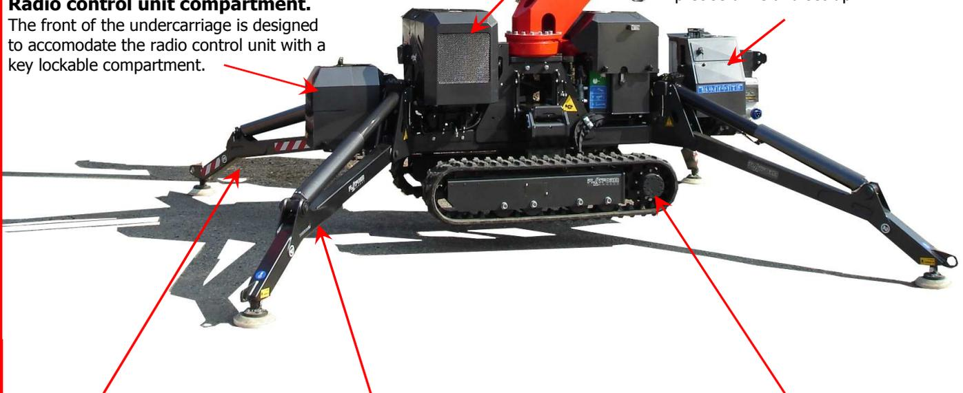
**Automatic stabilization set-up. (Self-levelling)**
